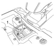
**NOTE:** Use of a non-standard pressure cap will not allow the recovery system to function properly. Contact your dealer for the correct replacement part.
